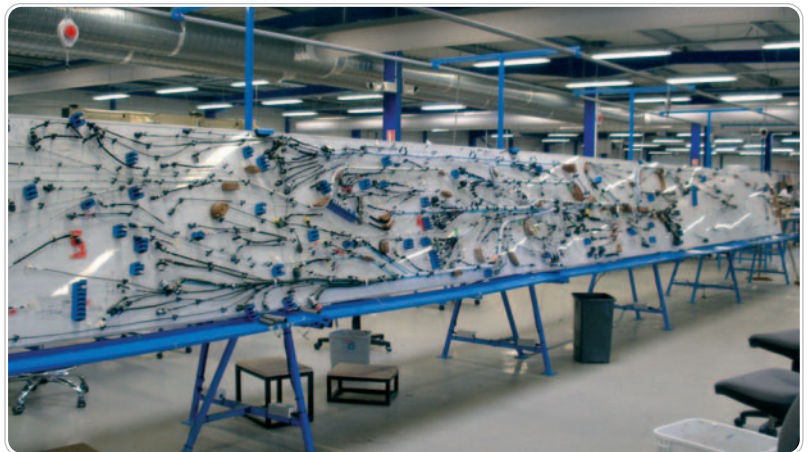
→ Falcon 7X harnesses manufacturing in Liposthey
